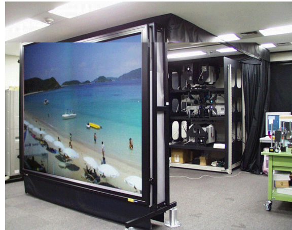
Fig.6 The photograph of 2x2 tiled 6-primary projection display system used in the experiment.
