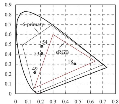
**Fig.4 The color gamut of six-primary DLP and sRGB display on CIE xy chromaticity diagram. The color coordinates of the patches used in the experiment are also shown. (The numbers marked in the graph correspond to the ones in table 1.)**
