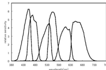
Fig.3 Spectral sensitivities of 6-band HDTV camera.
