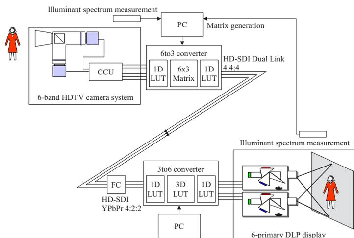
Fig.1 System configuration of the real-time video system using 6-band HDTV camera and 6-primary color display. FC:Format converter (4:4:4 to 4:2:2)
