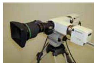
Fig.2 6-band HDTV camera.
